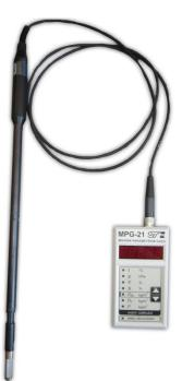
Every monitor is calibrated and thermally compensated within the range of 0 ÷ 40 °C. The pressure sensor applied guarantees accurate measurement and very good long-termed indication stability.
